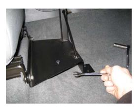
Tighten "Z" bracket to base assembly.
